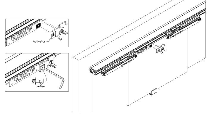
Step 7 Sliding the activator into the damper
