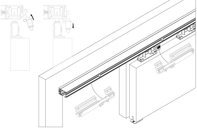
**Step 6**Fixing the activator to the wood holder
