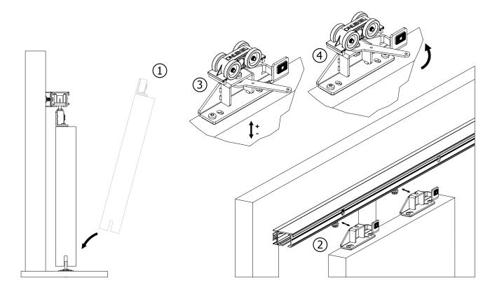
**Step 5**Swivelling the dampers into the guide rail
