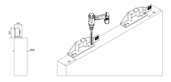
Step 3 Positioning the carriages in the wall-mounted running track
